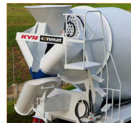
Staircase to inspection platform form is designed for operator comfort without compromising safety
